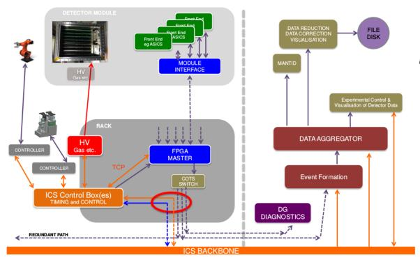
Data and control flow from a detector electronics perspective. The interfaces with the DMSC and ICS are indicated. How the data fits into the various aspects of the system are shown .
