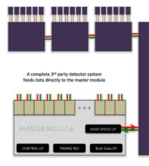
In this case the external partner supplies essentially a complete readout system for the detector array.
