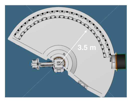
Last window: Monochromatic chopper Guide exit within sample environment area
