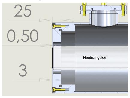
0.5 mm Al windows (Al 2024) FEA calculation show failure Yet in operation at ISIS. CSPEC will develop & test prototype.
