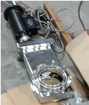
Valve to keep CCR sample area evacuated while installing SC
