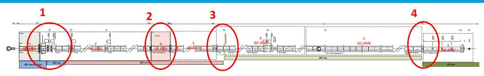
Differential movement at the junction between slabs (mm level)
