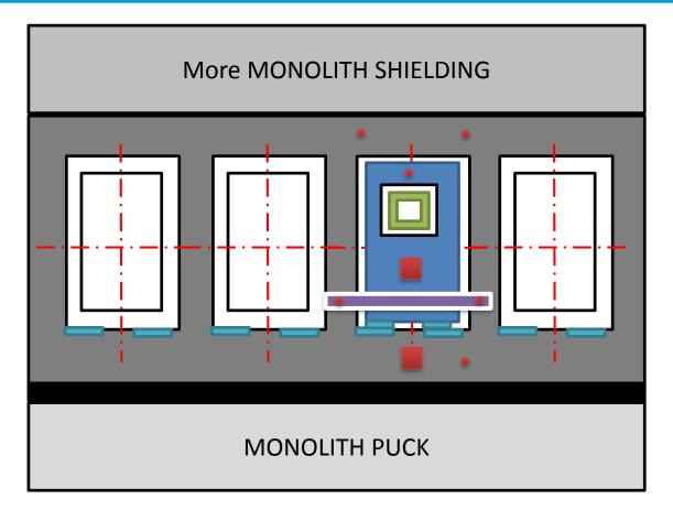
Real position on NBEX (thus NBOA) may be measured before BP Window installation and referenced with respect to BP reference features.
