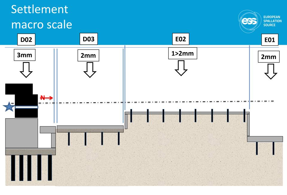
• Buildings settle onto foundations (piles or soil)
