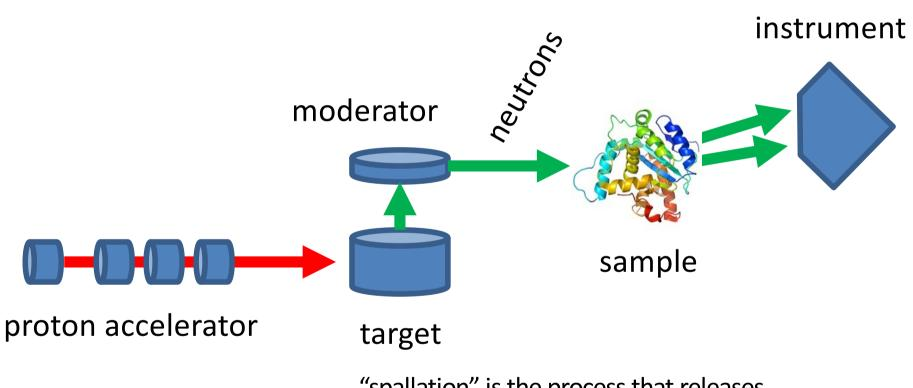
"spallation" is the process that releases neutrons from the target nuclei Neutron Production Target with innovative flat moderator design
