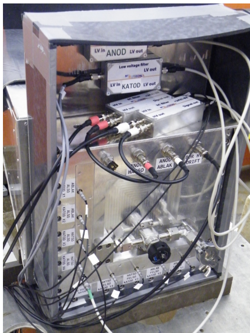
Solid boron converter neutron detector for source imaging
