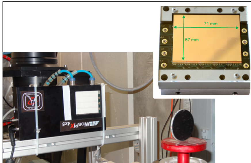
Large area Timepix detector Widepix4x5 covered with 6LiF
