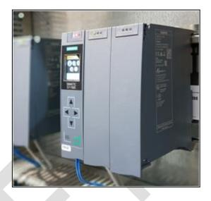
The inherent diagnostics functionality integrated into the SIMATIC S7-1500 system ensures that error messages are visualized identically as plain text information. The configuration and the diagnostic reporting channels are integrated into the system in a user-friendly manner. The trace function is supported on all CPUs. If a fault occurs, the corresponding channel can be quickly identified and precisely assigned. That reduces downtimes and increases availability of the cooling equipment.
