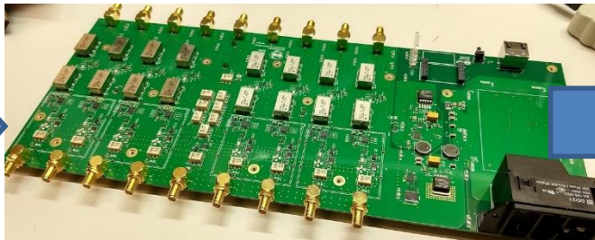
RFFE unit for calibration, filtering and gain
