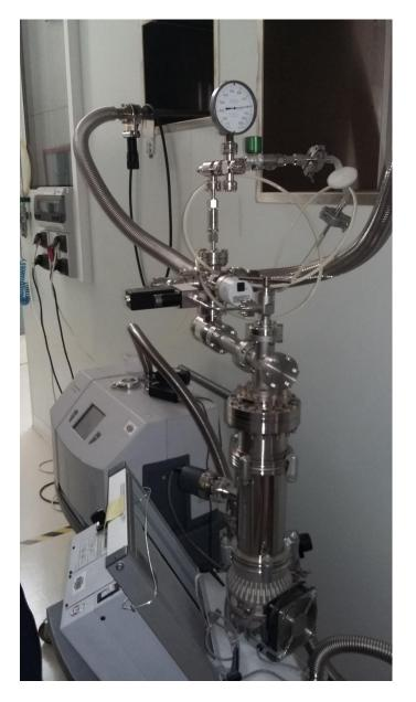
Slow pumping system and slow  $N_2$  filling up to atmospheric pressure developed by DACM staff member for compliance with free particle requirement.
