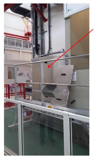
Gateway to access to big ultrasonic tank: The entire IPMs will be plunged in the bath and cleaned with specific detergent (TDF4, pH 13.5).
