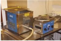
A- ultrasonic bath for cleaning + filtered water 534/1
