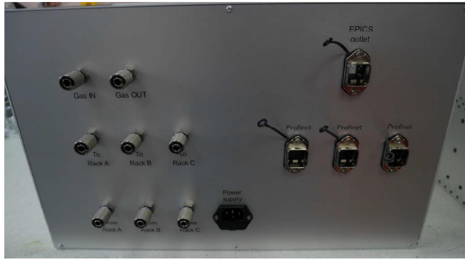
View of the back panel with the electrical connections and output of the distribution gas lines.
