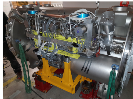
Figure 2: Prototype TCLD installed on the cryo-bypass (surface workshop)
