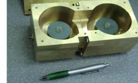
High quality filter for 1300 MHz, bandwidth 360 kHz (0.028%), IL=1.5 dB, thermal stability 2 ppm/°C, designed for DESY, Germany
