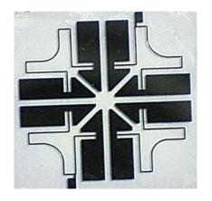
HTS YBCO filter on sapphire substrate for 2450 MHz, bandwidth 60 MHz (2.5%), size 8x8 mm designed for IF PAN
