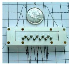
Waveguide filter for 22 GHz, size 50x13x10 mm, designed for MWTG, Canada
