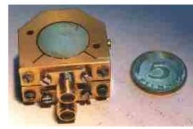
HTS YBCO dual mode waveguide filter for 3900 MHz, bandwidth 40 MHz (1%), size 22x22x10mm designed for Bosch, Germany
