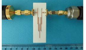
Waveguide diplexer with low pass input for 13 GHz, size 150x85x15 mm, designed for MWTG, Canada
