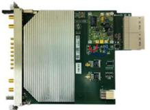
1.3GHz Vector Modulator developed for DESY/Struck GmbH
