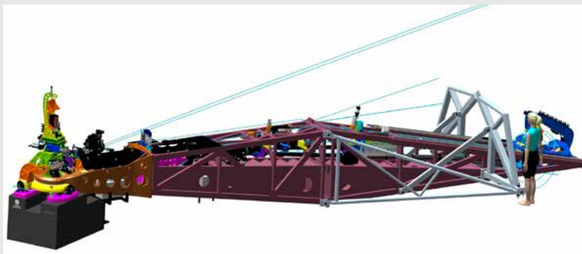
The extremely advanced spectrometer arm at Veritas is one of many results of successful collaborations between MAX IV and the various Swedish universities. The set-up was designed and built at Uppsala University and is now being put into operation on the beamline. Illustration: Carl-Johan Englund
