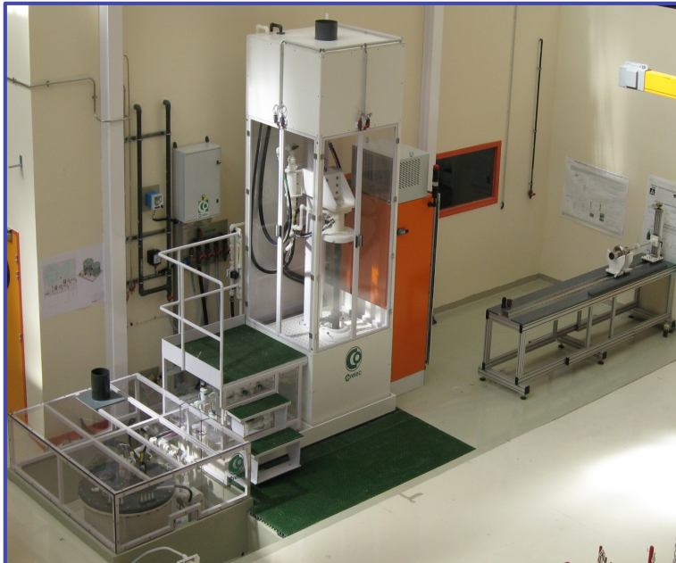
New Saclay vertical EP station: commissioned with 1.3 GHz single cell
