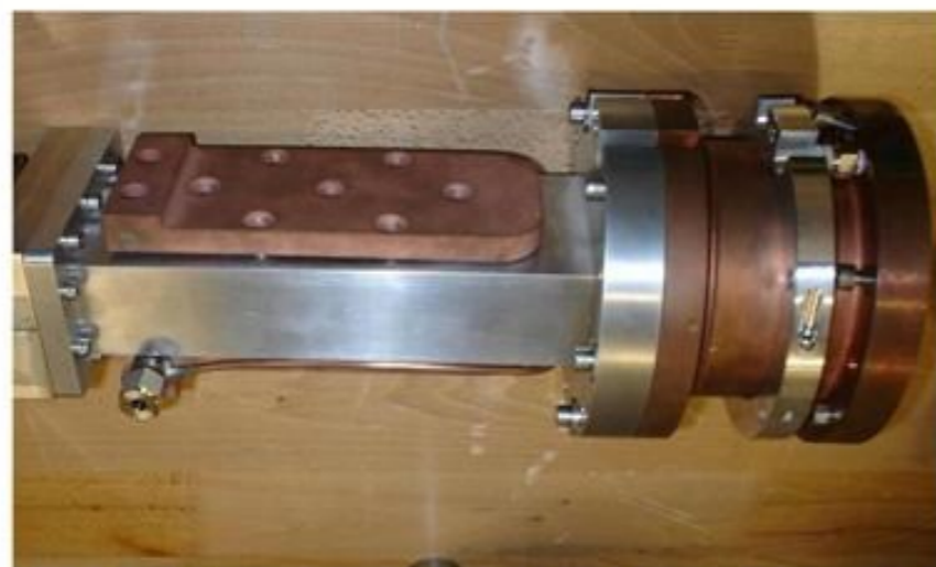
Matching transformer coupled to the plasma chamber
