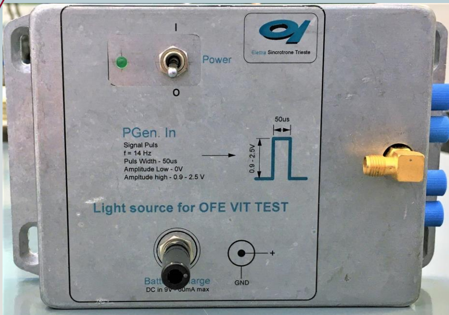
Equalized OFE optical tester
