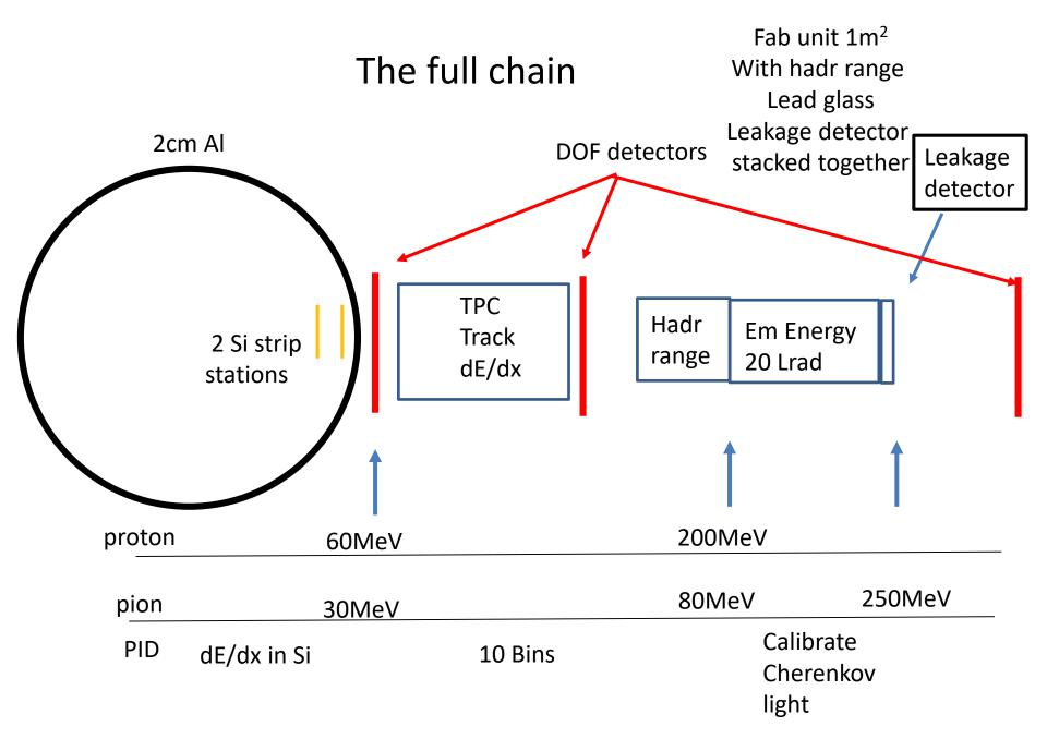
DOF detectors and cosmic charged particle veto . Plastic scintillators thick enough to separate MIP from gamma.
