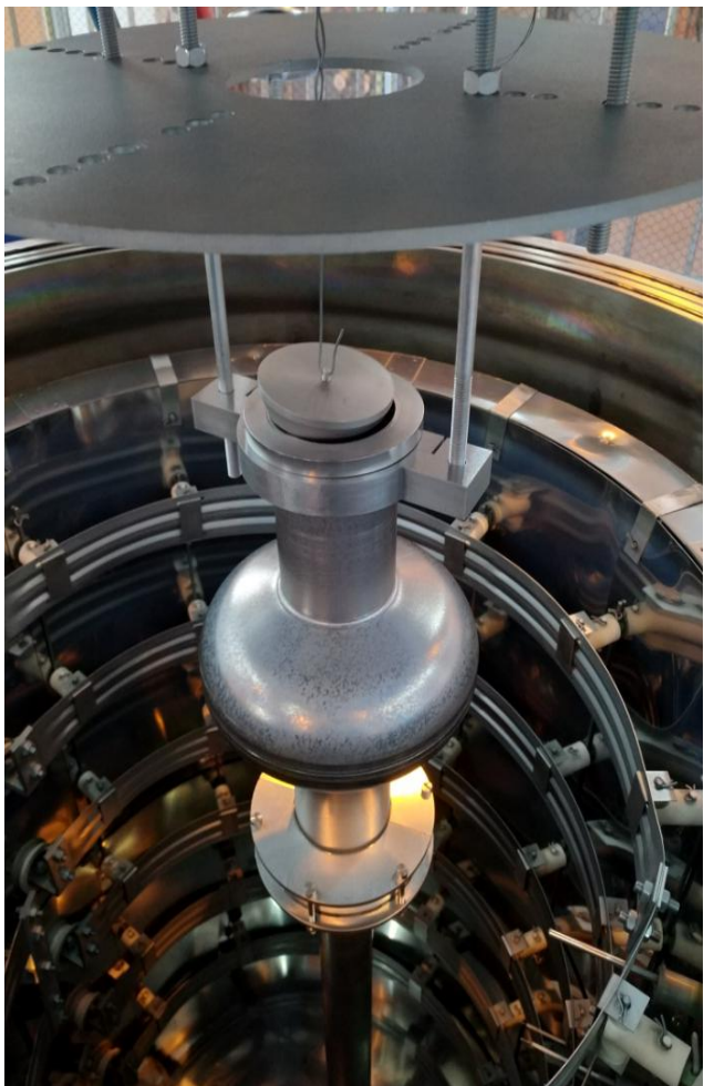
Nb 3 Sn on Nb cavity underwent 100°C 48h baking. Vacuum was kept below 1.4e-5 Pa
