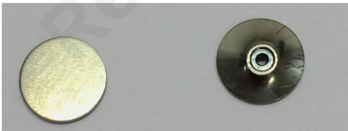
Figure 18 DAC gaskets. On left is a new un-indented gasket, which has a diameter of 6mm and thickness of 400 \mu\text{m} . On the right is an indented and drilled gasket. The alignment mark is seen at approximately 1 o'clock. Not that, in addition to the indentation, the gasket is seen to cup downwards.
