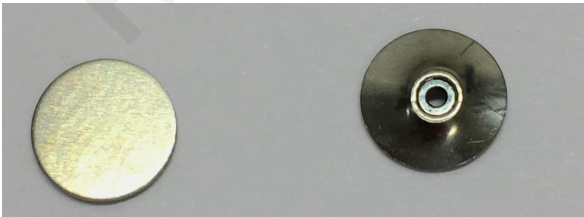
Figure 16 DAC gaskets. On left is a new un-indented gasket, which has a diameter of 6mm and thickness of 400 \mu\text{m} . On the right is an indented and drilled gasket. The alignment mark is seen at approximately 1 o'clock. Not that, in addition to the indentation, the gasket is seen to cup downwards.
