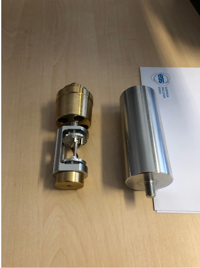
Figure 1 Huginn vacuum can for VTI sample stick
