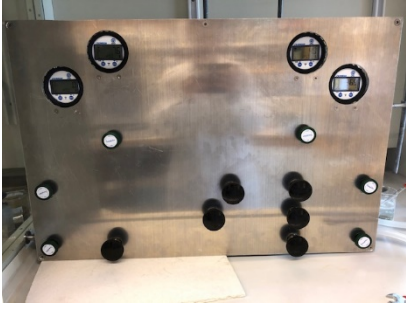
Figure 1: Gas handling manifold. Front view (left) and back view (right).
