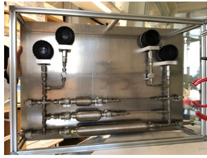
Figure 1: Gas handling manifold. Front view (left) and back view (right).
