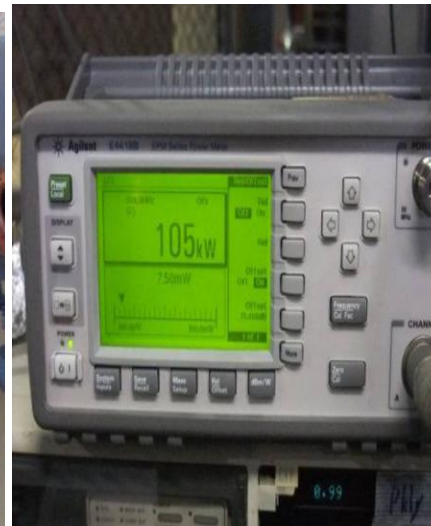
Window assembly high power test result: 100 kW, CW,TW
