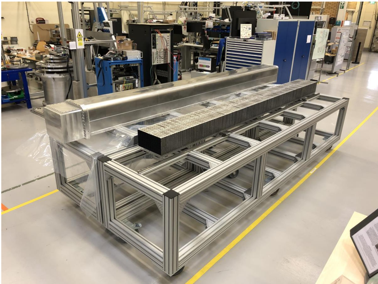
Figure 1. The prototype mechanical detector vessel for CSPEC in Utgård, Lund.
