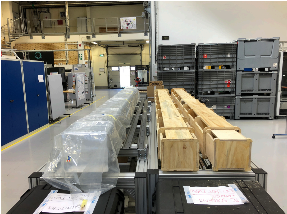
Figure 7. The wooden mockup vessels for CSPEC
