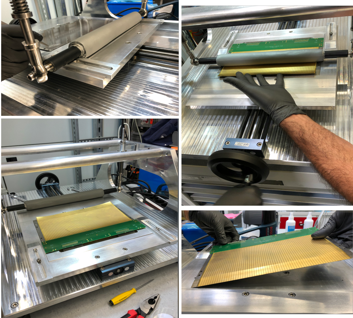
Figure 3. The assembly tooling for Multi-Blade: KV-1
