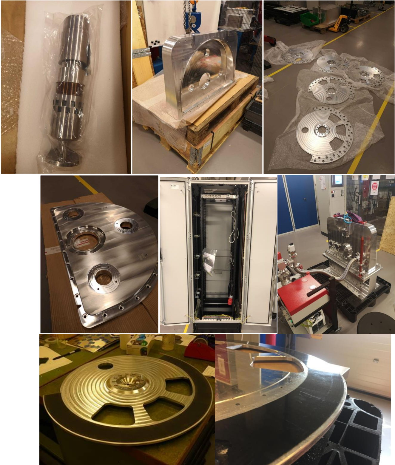
Figure 1. Fabrication of the first standard chopper as part of QA Phase. Top left: SKF Shaft with new Julich style disc coupling to be incorporated in the first QA phase chopper. Top middle: Upper chopper housing awaiting assembly. Top right: Uncoated test discs fabricated from 6082 and 7021 aluminum alloys (disc design based on a slow band chopper). Middle left: Upper housing cover plate. Vacuum and sensors ports as well as spindle fixation port visible. Middle middle standard chopper rack middle right Complete assembly QA phase chopper undergoing vacuum tests. Bottom left coated ISIS discs delivered Right: First inhouse coated NSS chopper disc
