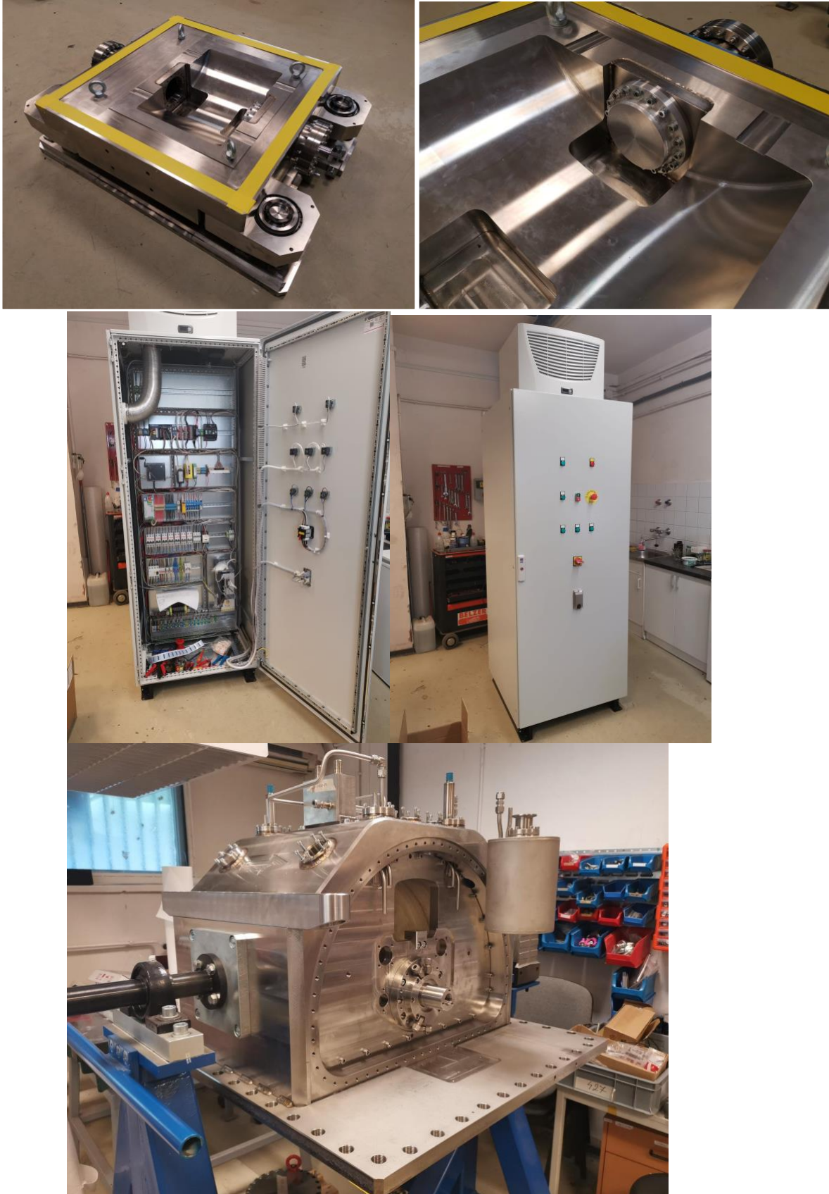
Figure 3. Fabrication of the 1 st T0 prototype fulfilling DREAM & T-REX specs. Top Left: Bottom T0 housing with Z-alignment features in each corner. Top Right: Detail of internal flange option for vacuum separation of T0 from guide vacuum. Bottom left: Top housing of T0 after CNC fabrication completion. Bottom Right: Control cabinet in
