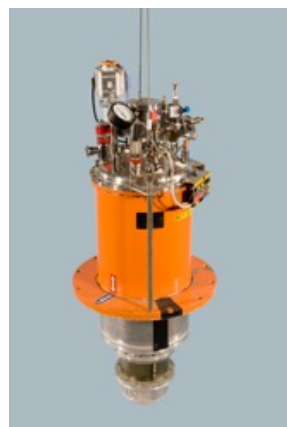
cryofurnace 1.5K-600K (800K)
