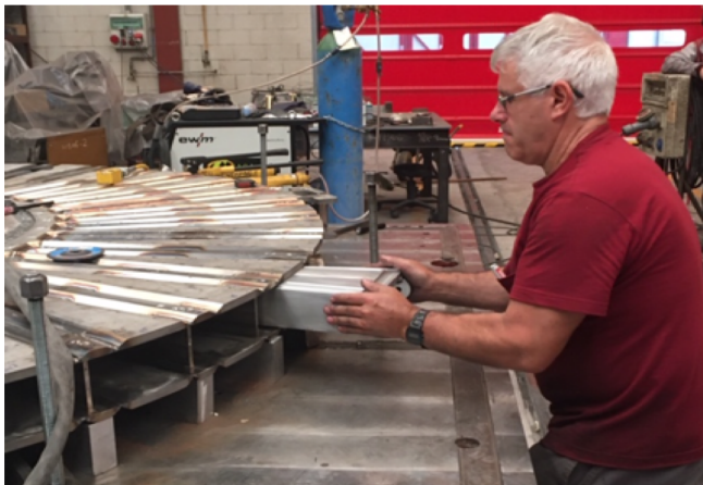
Target wheel ribs in place and tack welded. Tested with dummie cassette
