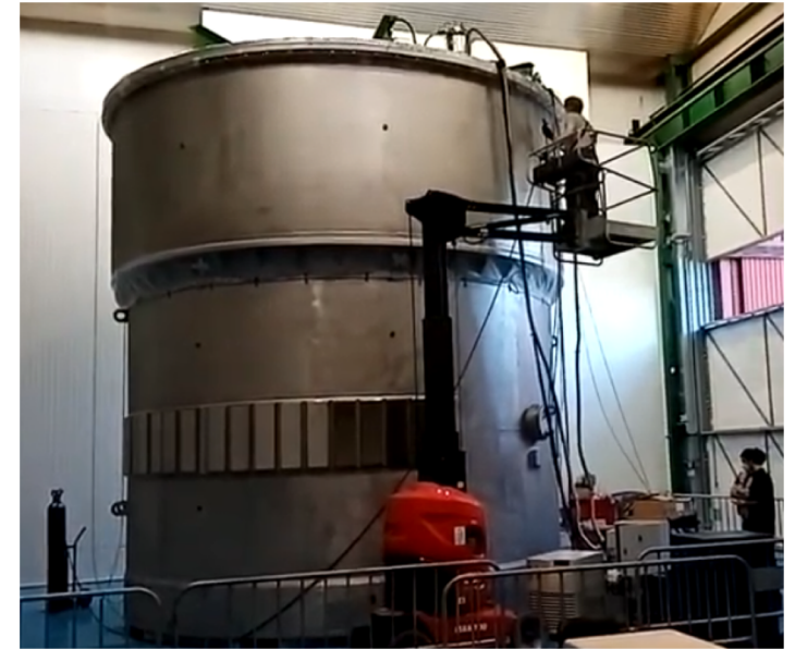
Monolith Vessel, lower & mid parts – in final machining steps, Delivery Oct 1
