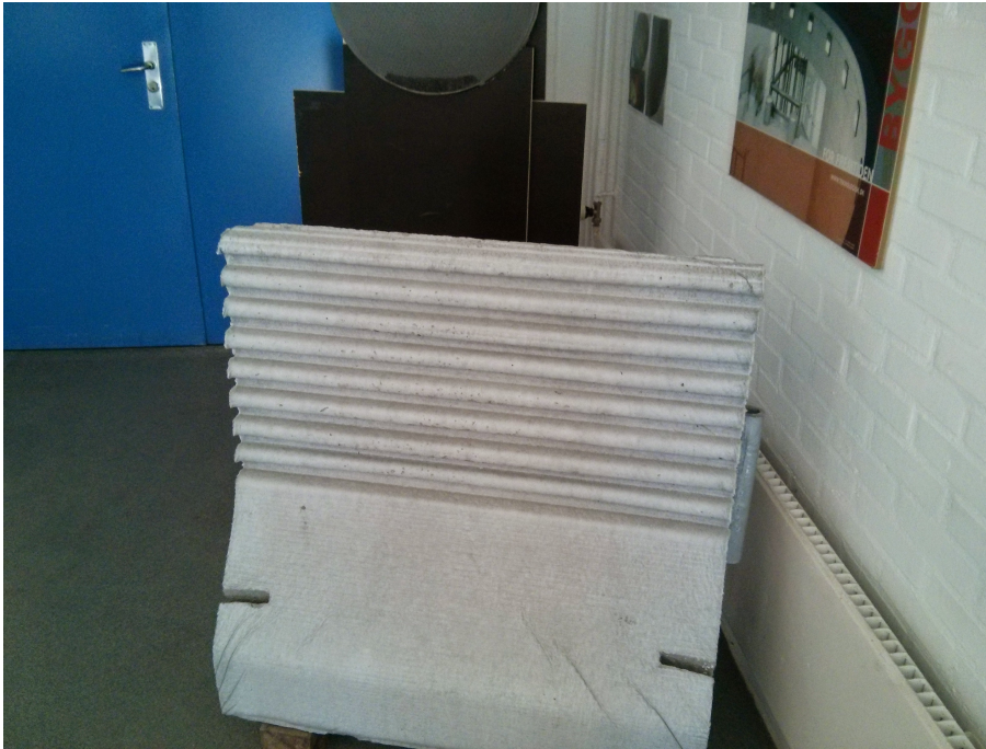
Figure 4: Concrete surfaces moulded for increased roughness. The waviness should be greatest along the beam axis, unlike this example shown here which is a decorative motorway barrier. Many thanks to DTI for this example.
