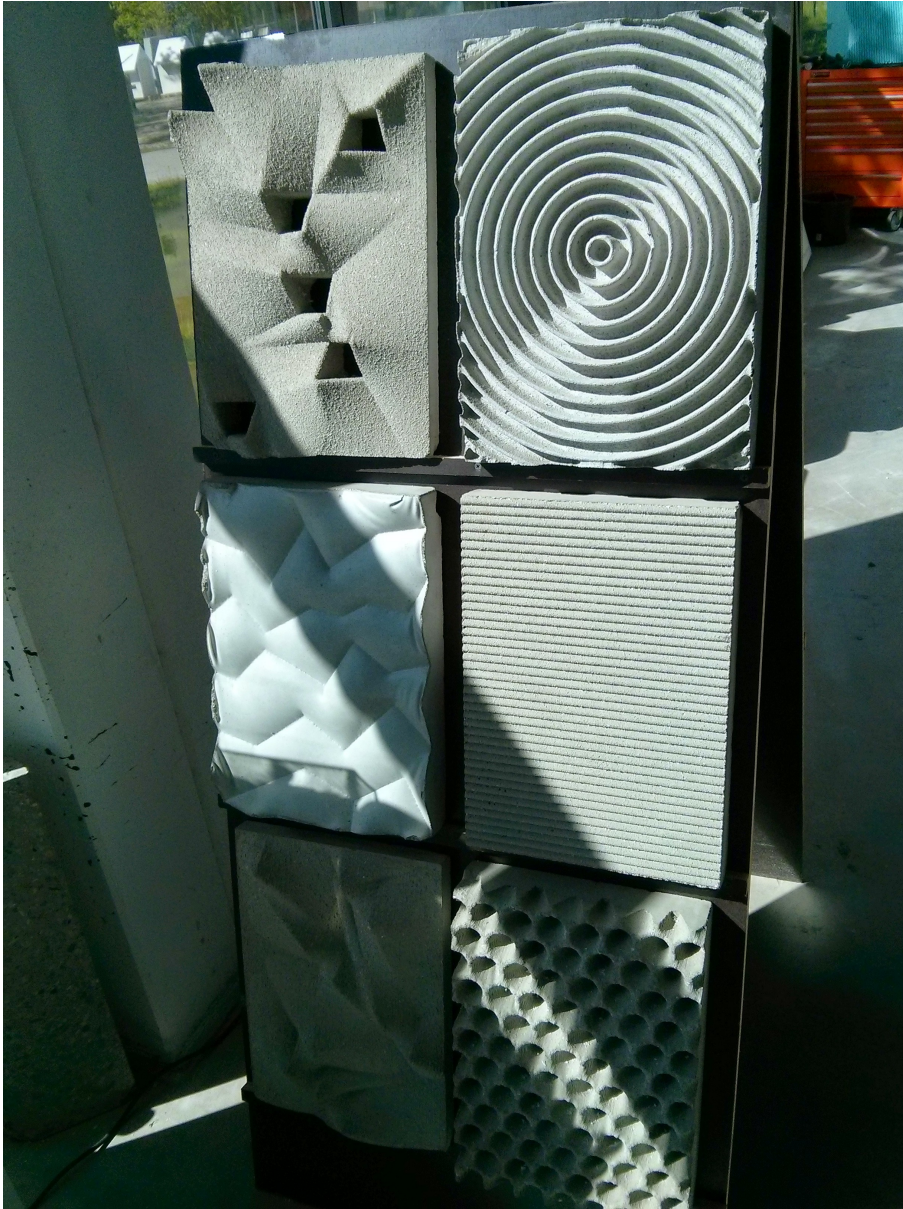
Figure 3: Concrete surfaces machined and providing increased roughness. The roughness should be greatest along the beam axis, unlike some of these decorative panel examples. Many thanks to DTI for this example.
