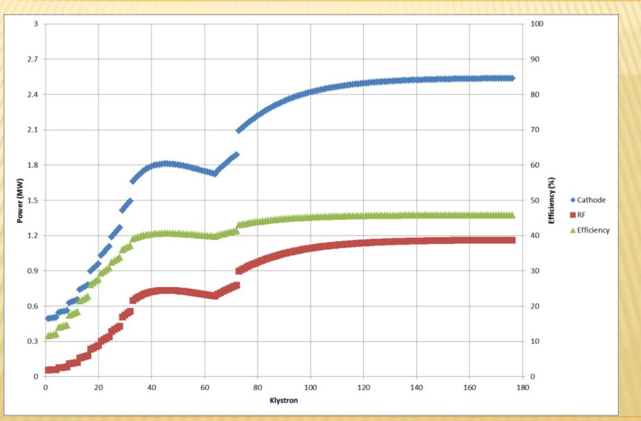
ESS Klystron Modulator Requirements
