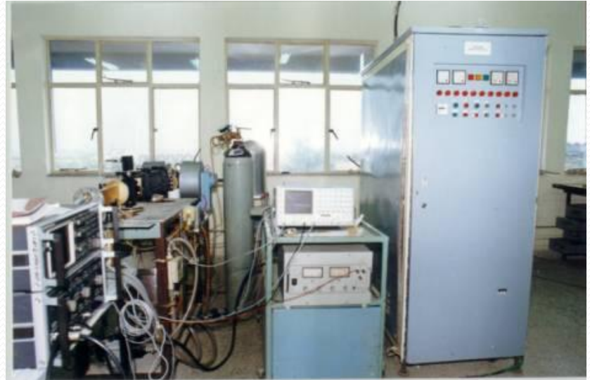
2MW MAGNETRON HIGH POWER TEST STATION DEVELOPED BY (RR)CAT
