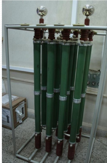
Dummy load of 5kOhms, 100kV, 17kW (without oil cooling) & 100kW with oil cooling. Oil tank not shown
