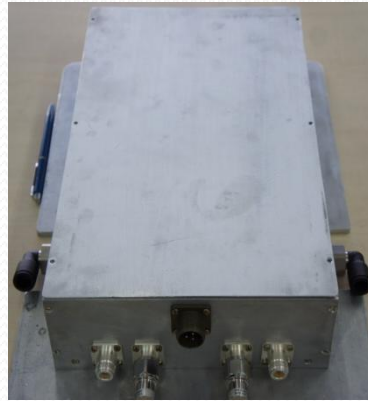
1.3 GHz 500W amplifier module assembly with divider/combiner
