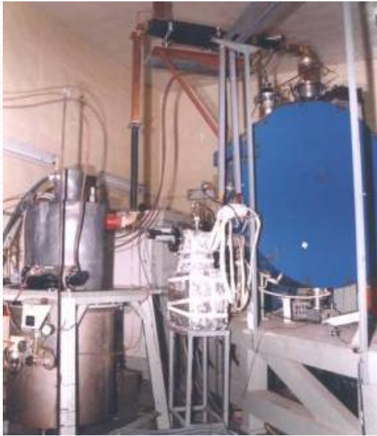
5MW peak power S Band pulsed klystron based microwave system for 20MeV Microtron pre-injector for Booster Synchrotron of Indus 2
