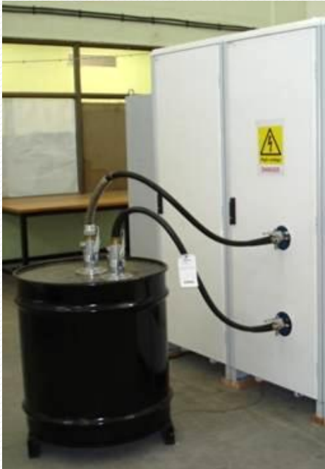
Modulator output connected to Dummy load of 5kOhms, 100kV, 4kW
