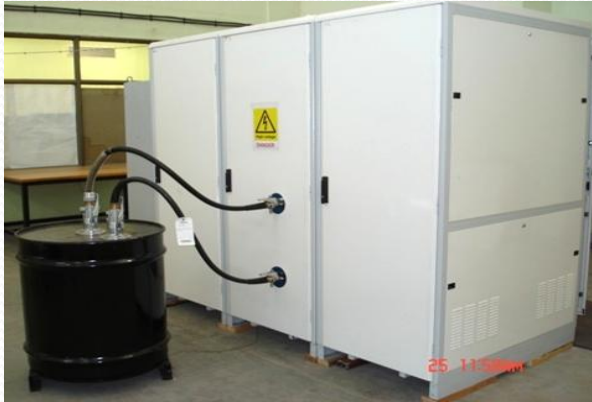
Modulator connected to 110kV resistive load
