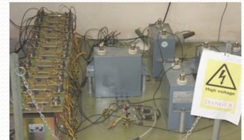
Tests on Marx cell with droop compensation networks
