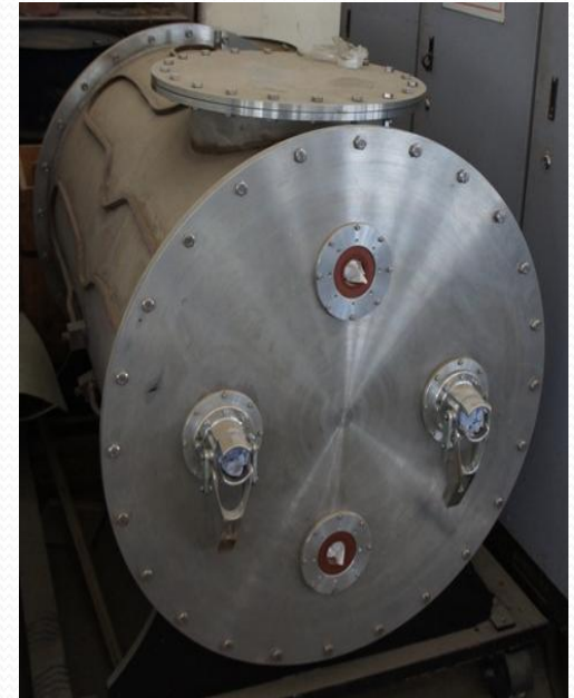
Load of 5kOhms, 100kV, 40kW with water cooling
