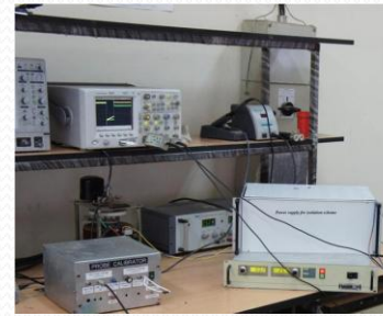
Tests on Marx cell with droop compensation networks
