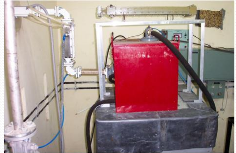
6MW Klystron with X ray shield connected to waveguide line to LINAC
