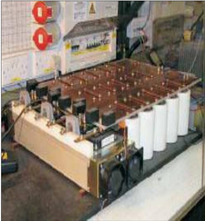
H-Bridges and DC-link capacitors
