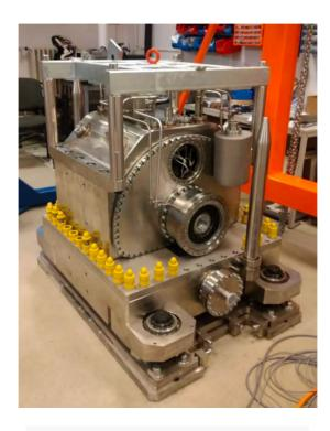
Prototype T0 chopper design speed of 31Hz reached
