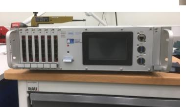
Back End Electronics - 5 Master Module readout crates in assembly as prototypes
