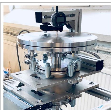
Figure 3: Fatigue testing of vacuum window.
