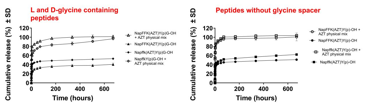
Burst release significantly reduced in chemically conjugated vs. physically mixed zidovudine (AZT): 40-50% in first 72 hours
