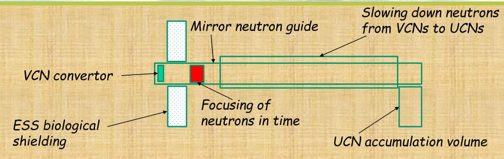
The VCN converter is installed in the region of the maximum neutron flux in the neutron source and might be surrounded on all sides, except for the direction of VCN extraction, by a nano-diamond reflector, transparent to thermal and cold neutrons, but completely reflecting VCNs.
