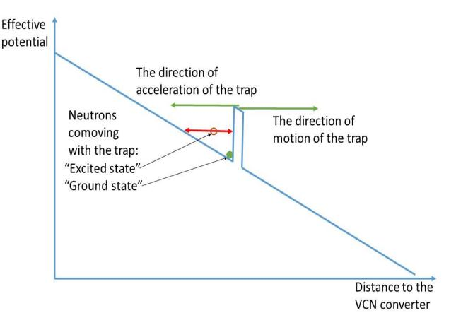
**Effective potential trapping the neutron bunch** in the coordinate system associated with the escaping slowing down trap
