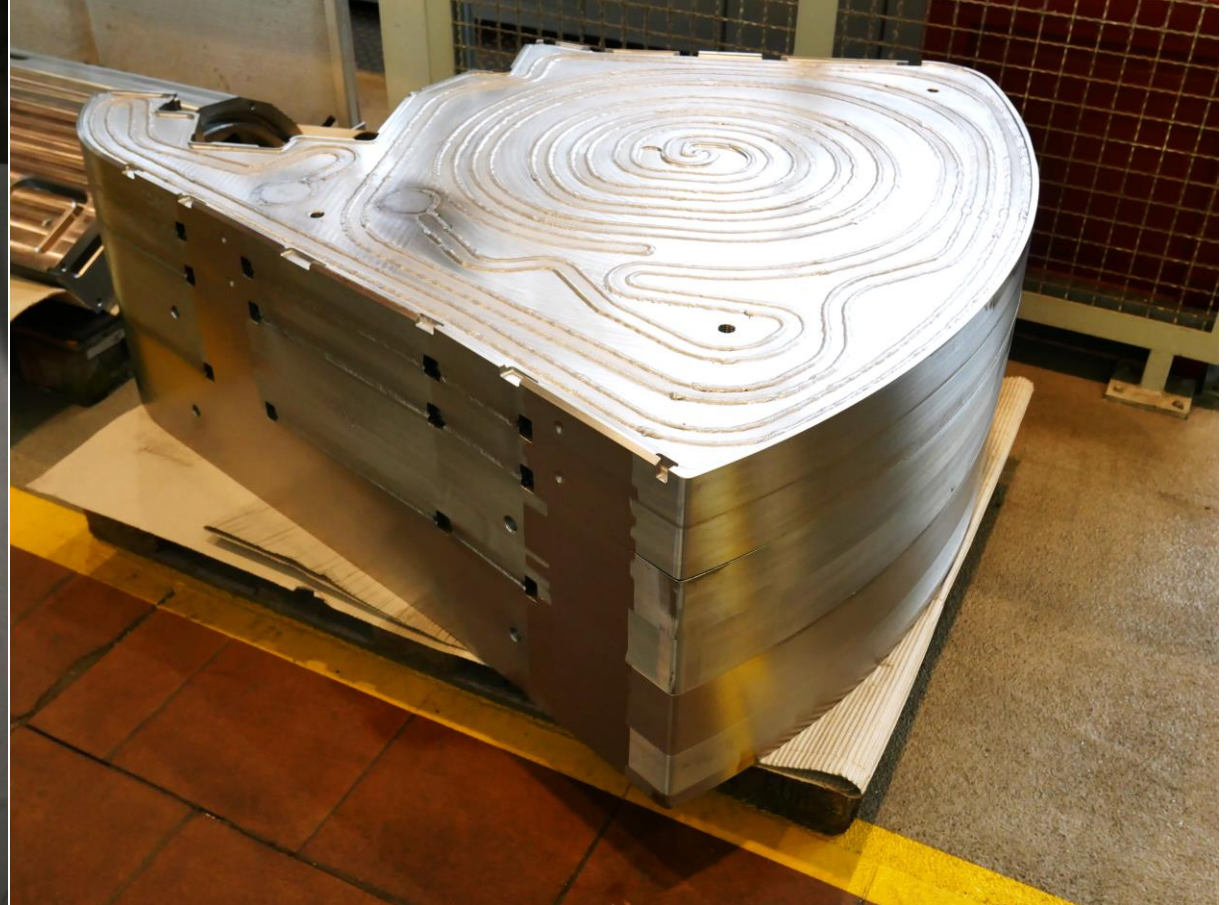
Lower Moderator Plug replacement
