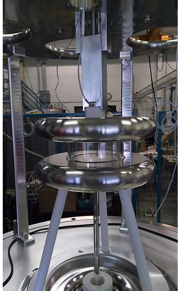
HV discharge testing of electrodes, insulators, coatings, comagnetometer gases.
