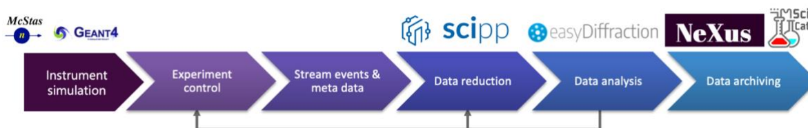
Figure 1: The DMSC data pipeline. Each chevron corresponds to a class of services needed for processing experimental data. The backward arrows show a mechanism to interact with the ongoing experiment based on feedback from the data reduction or analysis services. The software or frameworks are listed above the chevrons.
