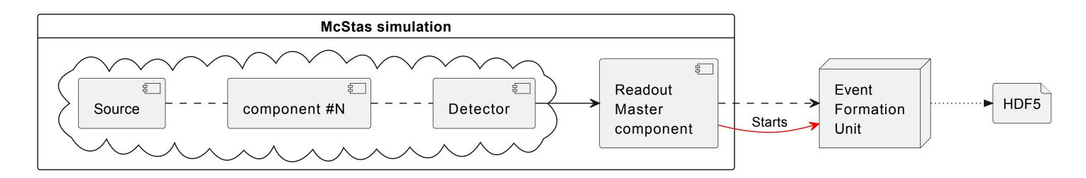
• Extending components allows appending (TUBEid, FENid, RINGid) to detected weighted neutrons
