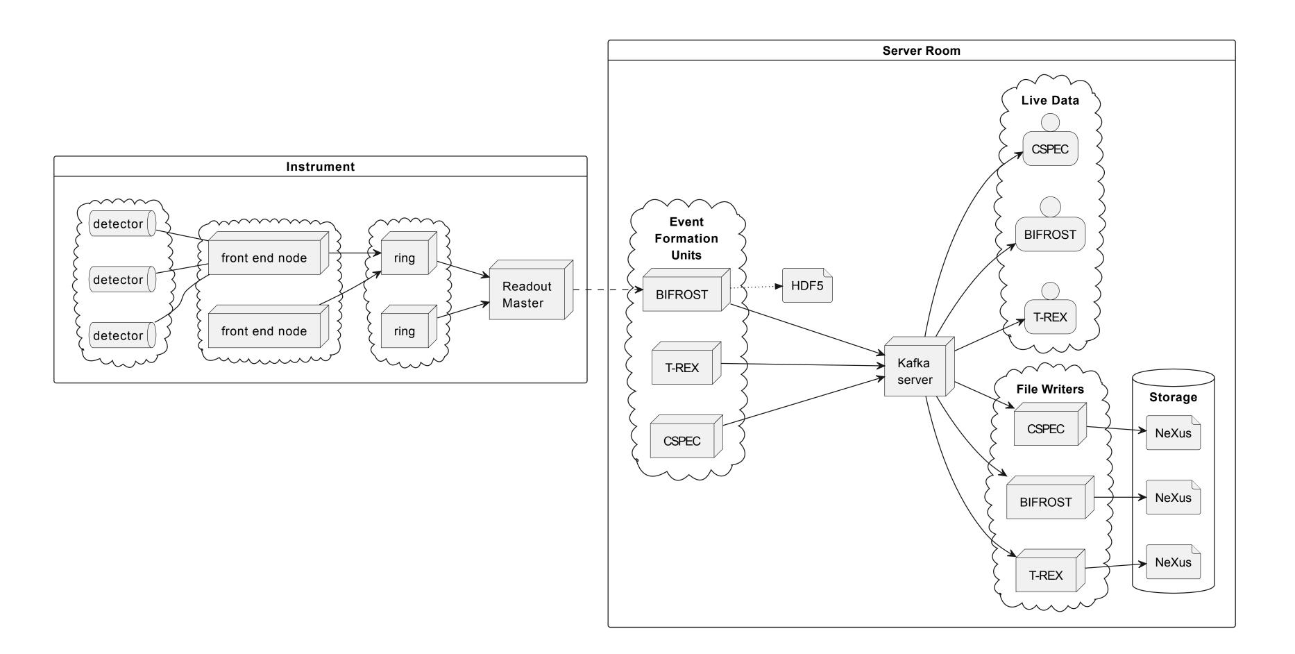
The Event Formation Unit converts this to (DetectorIndex, EventDeltaTime, PulseTime) where the index identifies a logical pixel in one of the continuous position sensitive tubes.
