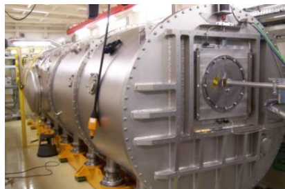
Tunnel under vacuum with X-rays detector
