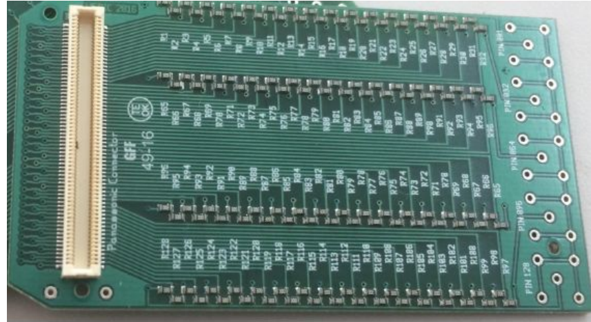
128 channels resistive chains
