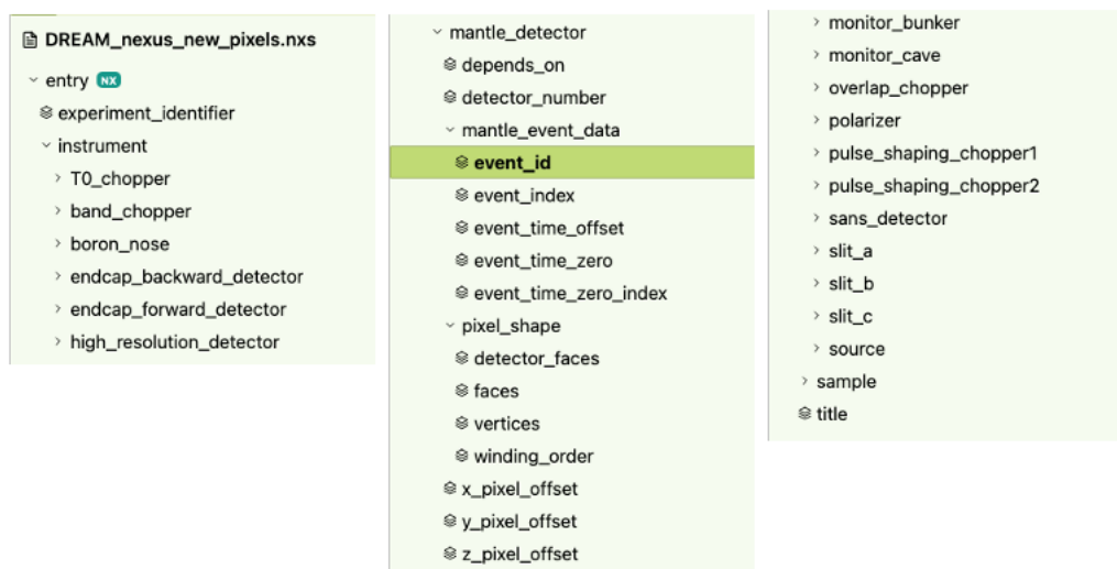
Figure 3: Tree structure of DREAM NeXus file showing the storage of different components of the instrument: slits, monitors, detectors, choppers. Note that the structure is displayed in 3 columns because of size constraints; but it should be read as a single entity. The detectors are split by banks: mantle, endcap backward and forward, high-resolution and sans detectors. The 2 nd column details the information stored for the mantle detector.
