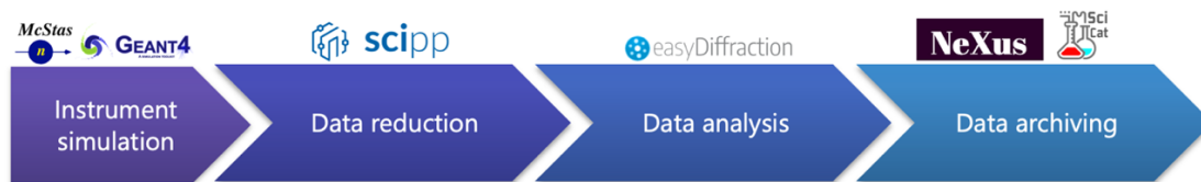
Figure 1: The data processing pipeline. Each chevron corresponds to a class of services needed for processing data. The software or frameworks described in Section 2 are listed above the chevrons.
