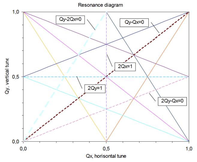
The operating point of the machine should be far from any resonances.
