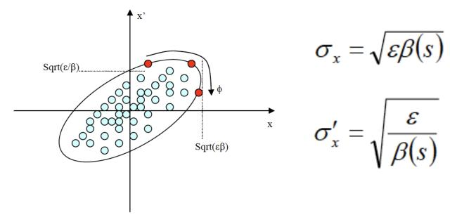
Large values of  $\beta(s)$  gives a large and parallel, non divergent beam Small values of  $\beta(s)$  gives a small and divergent
