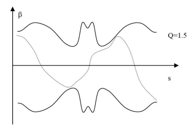
Betatron function and the path of an individual particle
