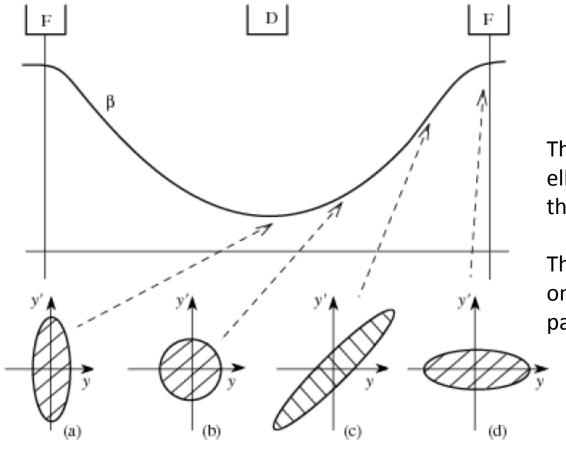
The tilt of the phase ellipse is given by the  $\alpha$ -parameter.
