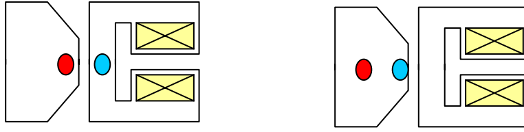
Fig. 9-7. Excitation of kicker magnets and rapid switch off before one turn is made.
