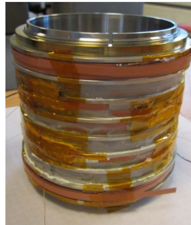
Coil with 8 sub-coils
