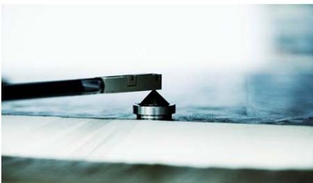
Alignment with magnet tip within 10 \mu\text{m}
