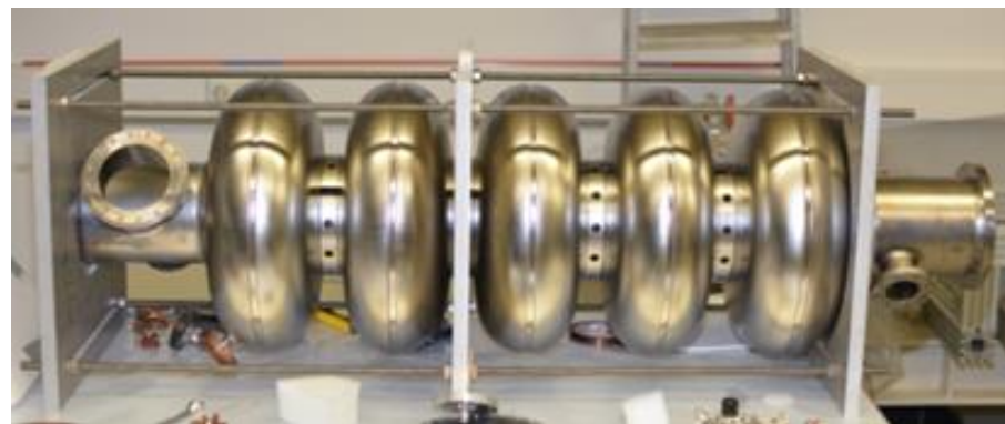
« ESS086-P02 » manufactured by RI F_{\pi} = 703.704 MHz Field flatness: 40% Bad angles stiffning rings
