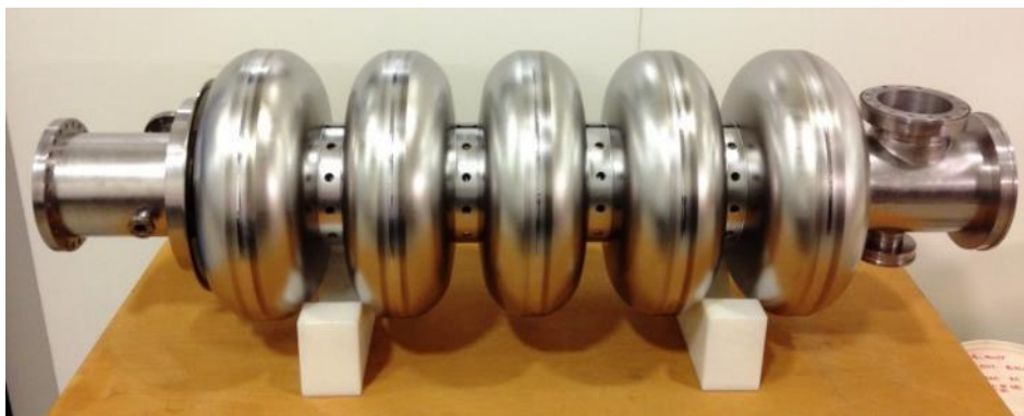
« ESS086-P01 » manufactured by E. ZANON F_{\pi} = 703.553 MHz Field flatness: 86%
