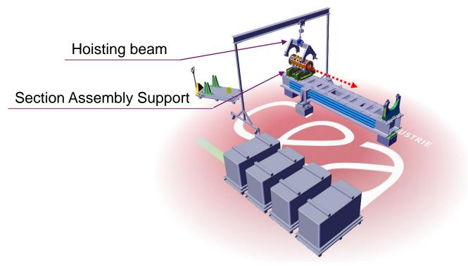
Section 1 is put in place on the Section Assembly Support sliding on the RFQ chassis.
