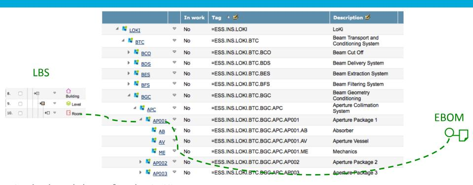
In the breakdown for the LoKI instrument you are able to go to the generic design, the EBOM, or to locate where its been installed, the LBS.
