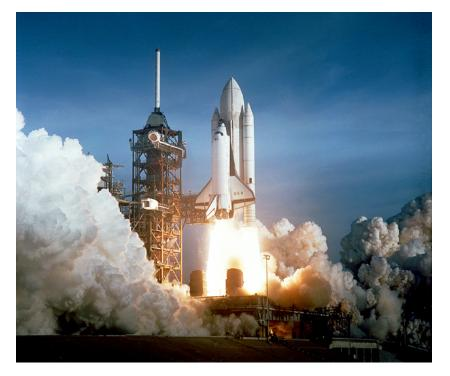
Main Shuttle Engines use LH<sub>2</sub> and LOX
