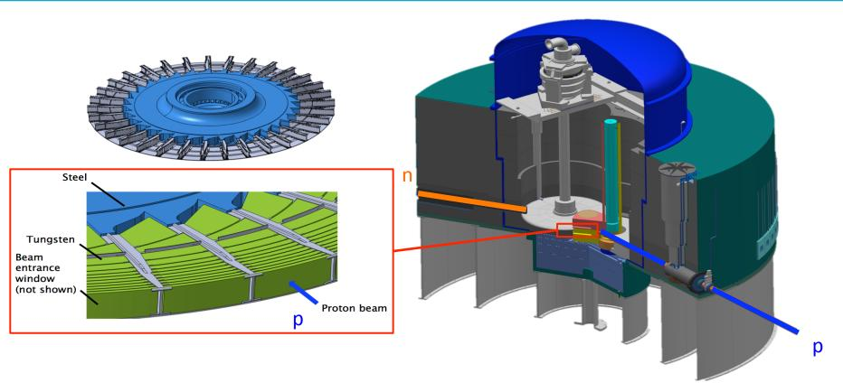
Target motion control system must be precisely synchronised with the 14Hz operation of the accelerator to ensure proton pulses can be 'painted' in the middle of the face of each tungsten sector.
