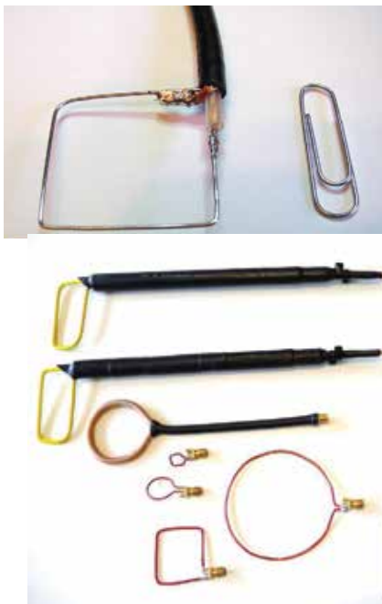
Near field probes, homemade above (Keith Armstrong)
